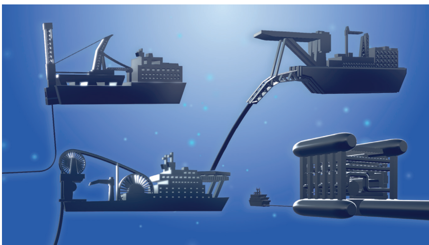
N'GENIUS CRA line pipe can be installed via J-lay, S-lay, Reel-lay and subsea Bundle installation techniques.
